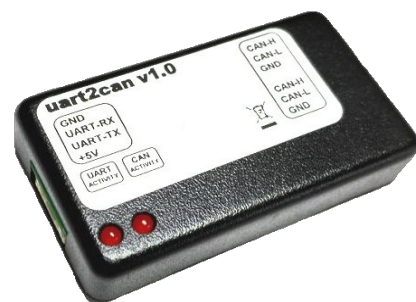
Figure 2.13: Tiny BMS UART-CAN communication module
